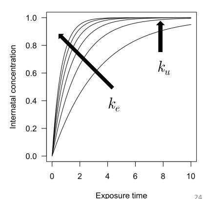
$$\begin{cases} \frac{dC_i(t)}{dt} = k_u \times C_w(t) - k_e \times C_i(t) & \text{if } 0 \le t \le t_c \\ \frac{dC_i(t)}{dt} = -k_e \times C_i(t) & \text{if } t > t_c \end{cases}$$
